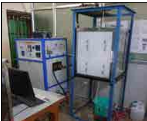
Induction heating based boiling test rig
