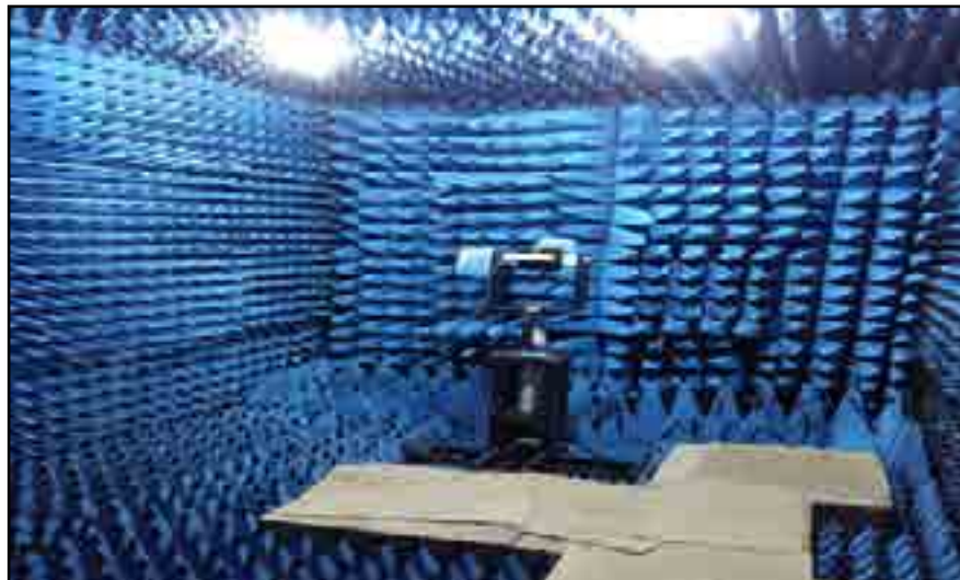
3. An “anechoic chamber” (“an-echoic” meaning non-reflective, non-echoing or echo-free) is a room designed to completely absorb reflections of either sound or electromagnetic waves. They are also often isolated from waves entering from their surroundings. (Anechoic Chamber with 6 axis position for RF Characterization (up to 20GHz))
