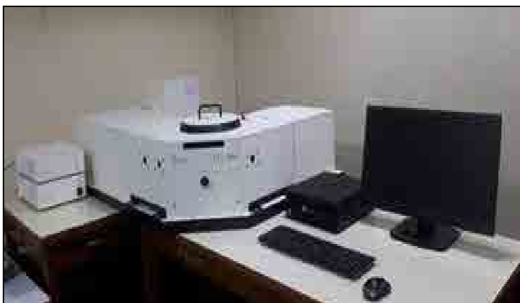
1. Photoluminescence (PL) measurement setup (F980) from Edinburgh Photonics, UK. This setup can provide PL from 200-800 nm.
