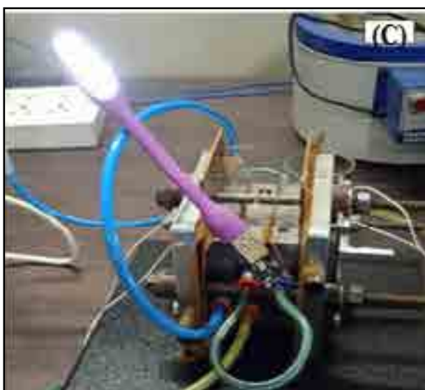
Fig. 1. Photographic view of (A) Unitized Regenerative Fuel Cell (URPEMFC) for the Production of ultrapure hydrogen (B) URPEMFC stack for hydrogen production in electrolysis mode and simultaneous power generation in Fuel cell mode showing LED light and (C) URPEMFC stack for hydrogen production in electrolysis mode and simultaneous power generation in Fuel cell mode showing array of LED light glowing with high intensity.
