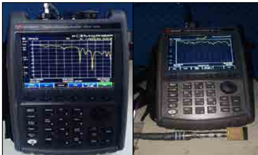
4. Handheld Vector Network Analyzer with measurement facility up to 44 GHz. The microwave characterization of the device under test can be performed at any location as the instrument is portable in nature.
