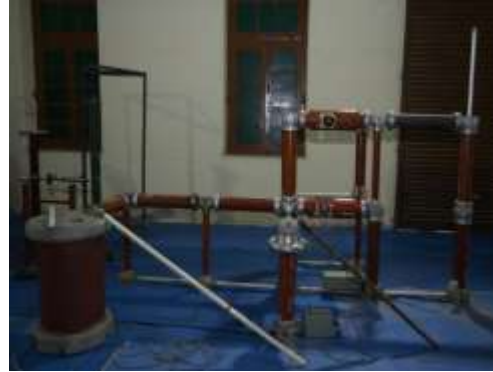
250 kV, 2-stage, Impulse Voltage Generator, WSTest System, Bangalore
