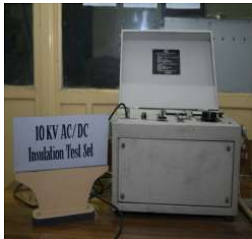
Insulation test set for transformer oil, Neo-Teletronics Calcutta
