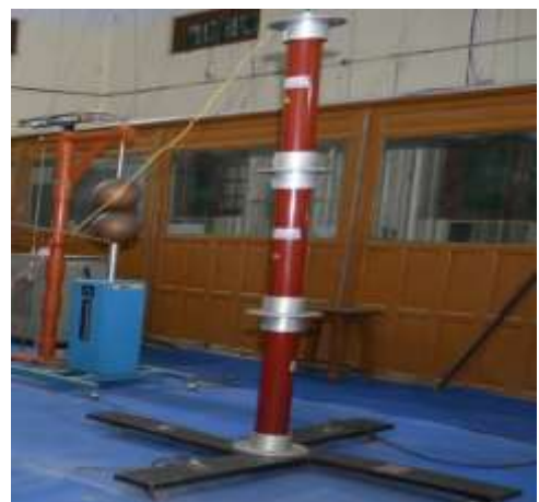
25 Cm Sphere Gap and 250 kV/250V and R-C Voltage Divider, Rectifier Electronics, New Delhi
