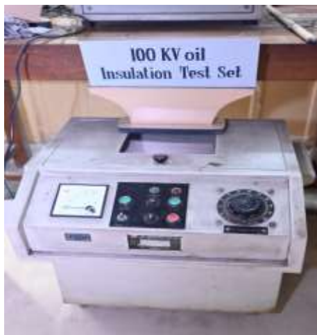
Insulation test set for transformer oil, Neo-Teletronics Calcutta
