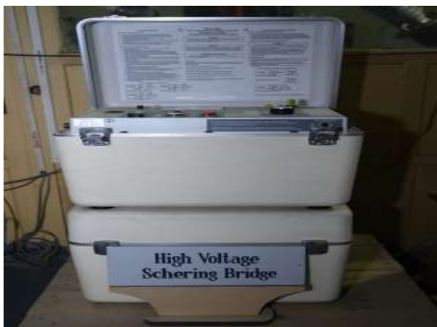
12kV Insulation Test set, Megger
