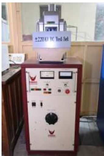
DC Dielectric Test set: 200 kV, 10mA, Phenix Technologies, USA
