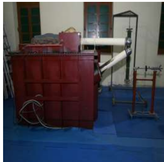
DC Dielectric Test set: 200 kV, 10mA, Phenix Technologies, USA
