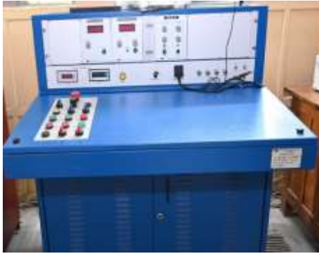
250 kV, 2-stage, Impulse Voltage Generator, WSTest System, Bangalore
