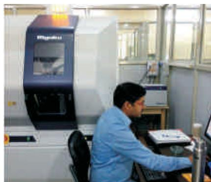
X-Ray Diffraction is a tool used to study the crystal structure of a material or confirm a single phase of a sample. It means XRD is the “finger print” of the material because it identifies which family of crystal structure, the structure of compound belongs to. When X-rays are scattered from a crystalline solid,
